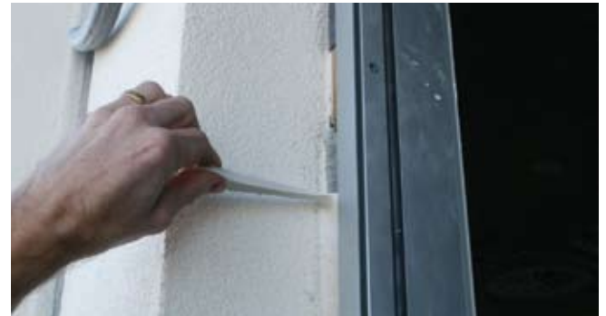
FIGURE 1.1 – ADHESION PULL TEST
