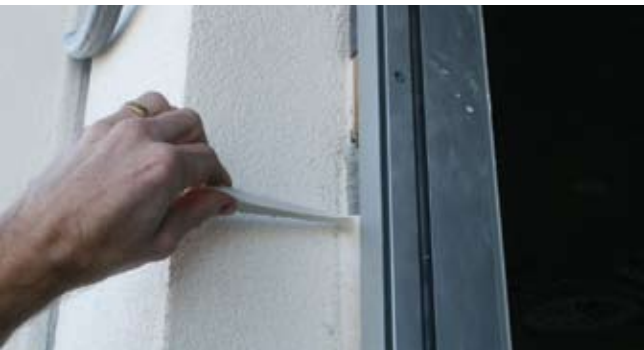
FIGURE 6.6 – FIELD ADHESION TEST
